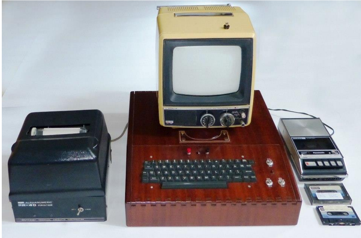
Apple I “system” with all original components: Datametics Keyboard STP PR-40 printer, Panasonic cassette player and cassettes with software; TV is 1975 Hitachi that connects via RF modulator that came to me with the Apple I – Rick Crandall collection
